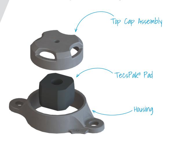
The TCC-45 LTLP-C is designed to operate at an installed height of 2-5/8" and provide 4,500 lbs. of preload and 5/8" of travel. It can also take the place of a friction block style bolster pocket when the 8.5-inch bolt pattern is available.
