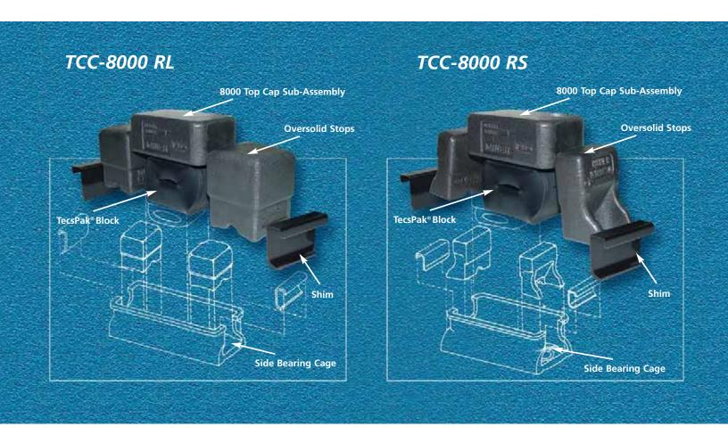
Designed to fit most 70 and 100-ton equipment, the TCC-8000 RL replaces the double side roller bearings in existing Stucki 688-B housing, while the TCC-8000 RS retrofit kit replaces the single roller side bearing in Stucki 656-C housings.
