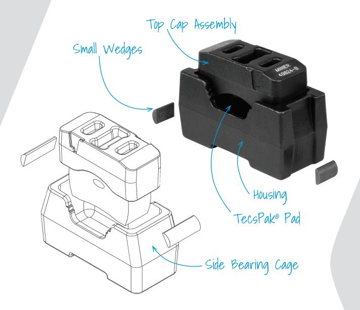
The TCC-45 LTRB is designed to operate at an installed height of 5-1/16" and provide 4,500 lbs. of preload and 5/8" of travel.
