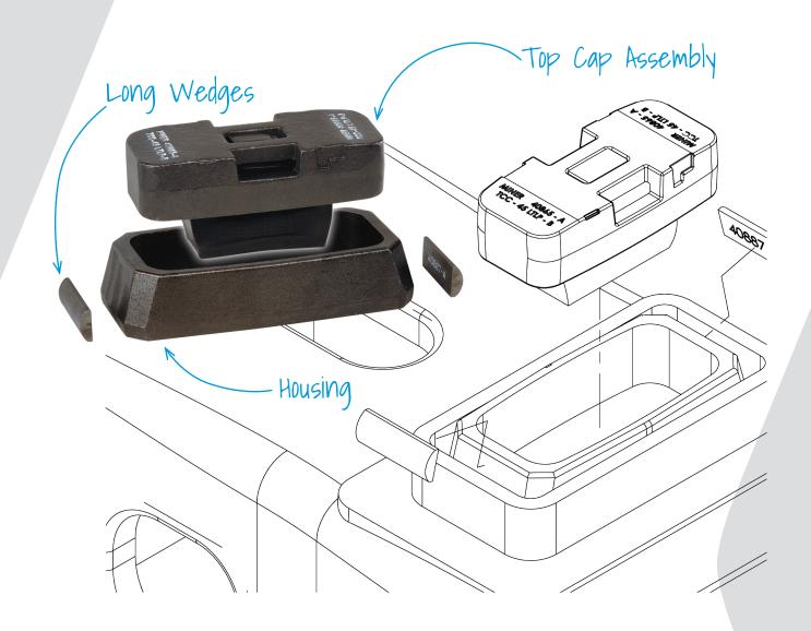
The TCC-45 LTLP-B is designed to operate at an installed height of 2-5/8" and provide 4,500 lbs. of preload and 5/8" of travel. The minimum pocket size to utilize the TCC-45 LTLP-B is 9-1/4" x 4-1/4".
