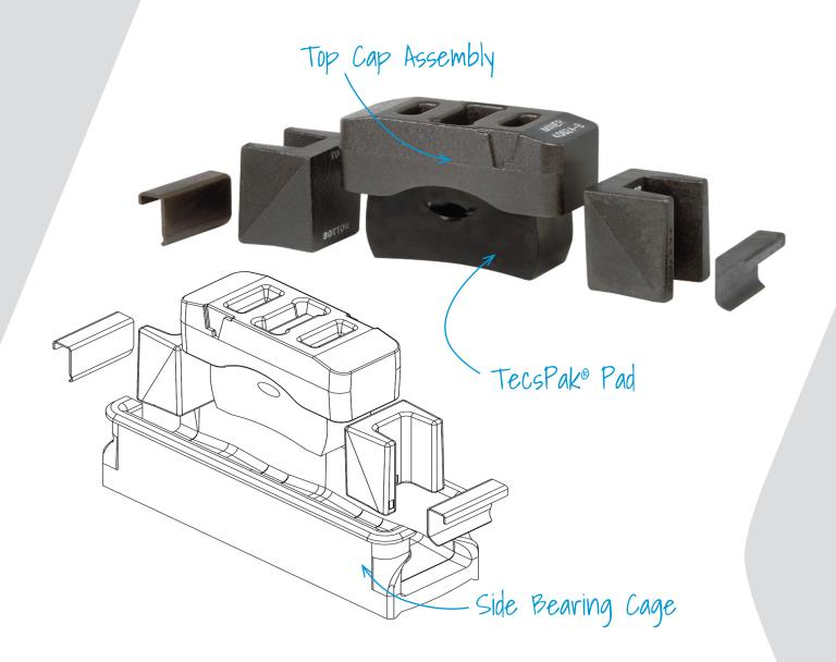
The TCC-45 LTR is designed to operate at an installed height of 5-1/16" and provide 4,500 lbs. of preload and 5/8" of travel. The TCC-60 LTR is designed to operate at an installed height of 5-1/16" and provide 6,000 lbs. of preload and 5/8" of travel.
