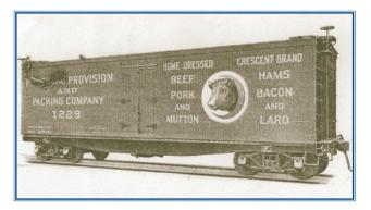
Refrigerator Car, Pressed Steel Underframe. Capacity, 50,000 lbs. Weight, 46,100 lbs. Length, 35 ft. 2-5/8 in. American Car & Foundry Co., Builders
