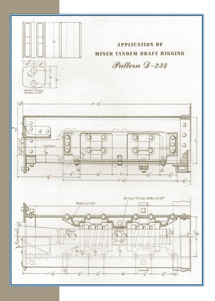
"The object of my invention is to provide a draft-rigging of a simple, strong, and efficient construction, embodying great buffing and pulling resistance, and providing for a gradual or cushioned absorption and transmission of strains and shocks to the body of the car.
