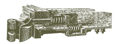
The deadly link-and-pin coupler shown at right was so arranged that the brakeman had to stand between the cars in order to achieve coupling. So hazardous was the job that brakemen were often identified because of missing fingers and/or crushed hands.
