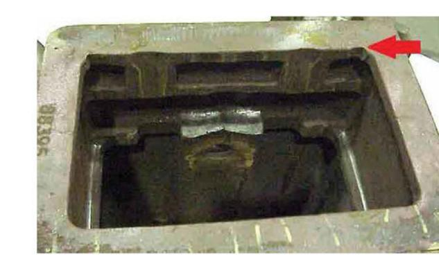
The visible depth of case wear into housing cannot exceed 1/4" (6mm) max.
