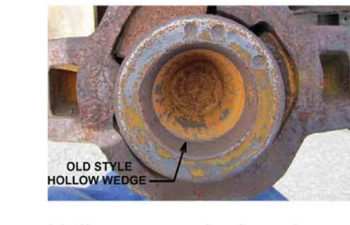
Hollow or cracked wedge.
