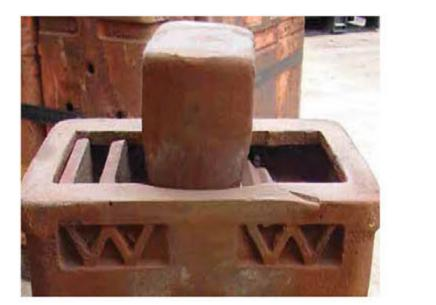
Non-critical areas with cracks 1" (25mm) or longer.
