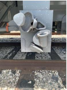
The lock handle is not required to touch the angle stop. The angle stop is there to prevent over-rotation of the lock handle. The images show full engagement of the operating handle in primary lock position. The lock handle is rotated to a position that wedges into contact with the operating handle.
