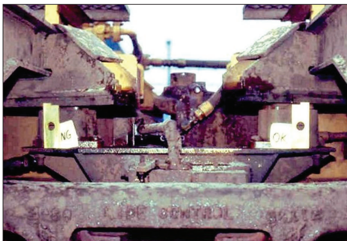
Figure 5. Articulated connectors have multiple surfaces that wear and can cause one side of the connector to drop in relationship to other. This reduction in height is transferred to the side bearings on the male side of the connector.
